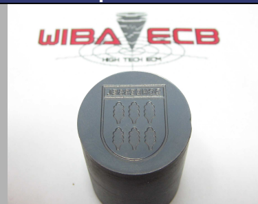
Powder metallurgic steel with only one electrode - tolerance 10 \mu\text{m}
